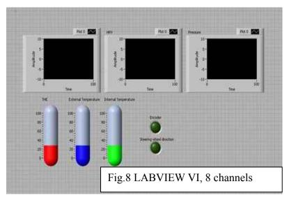
All the signals are acquired and digitized. In order to handle the signals a LABVIEW VI has been created [20, 21]. This VI acquires all the sensory data and checks them to ensure all sensors are properly working. Using the data provided by the sensor's manufacturer, regarding the sensor's
