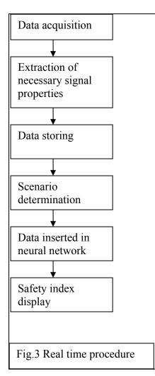
The purpose of the system is a real time evaluation of the driver's safety. Since only a very small amount of time is required for an incar situation to become dangerous, the system is evaluating the driver's state continuously.
