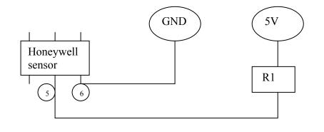
Fig.7 Circuit used to measure voltage instead of resistance
