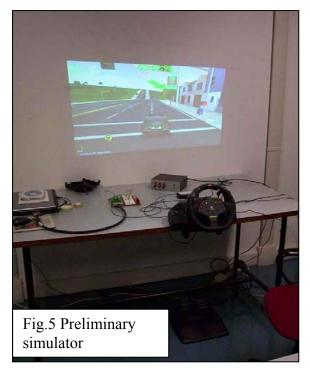
A preliminary simulator system has been developed at the Robotics Lab of the Politecnico di Milano. The system consists of a computer games' steering wheel with pedals and a computer game that is projected in front of the driver giving him the impression of actually driving.
